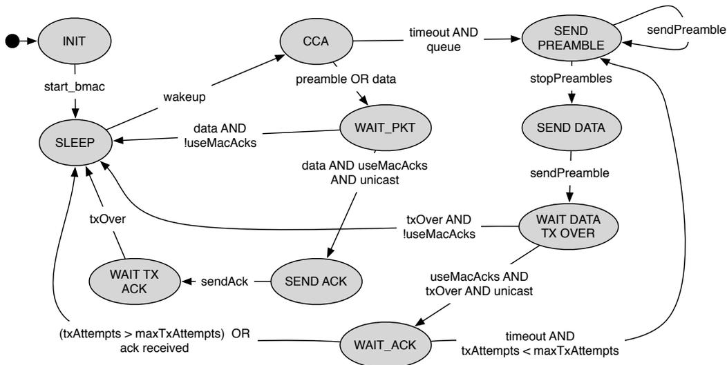
Figure 2: Finite state machine of the MiXiM implementation of B-MAC.
