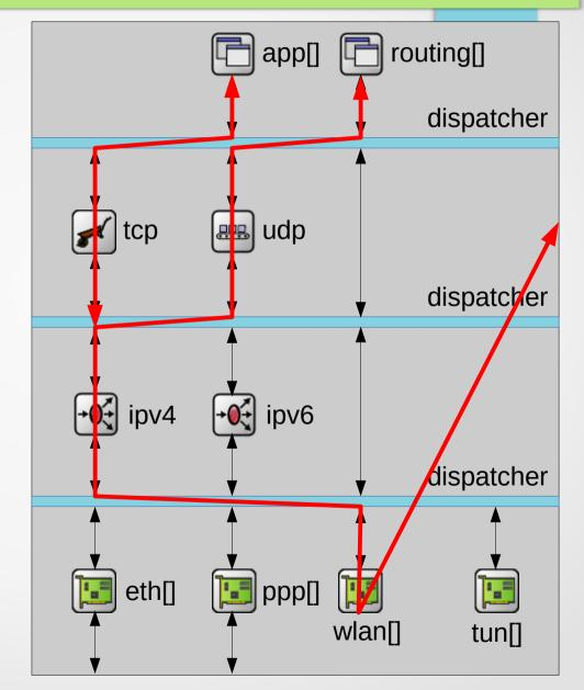
Tunnel application simultaneously opens a TUN device and a raw IPv4Socket
