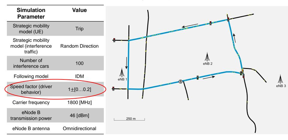
Sensing of the LTE signal strength using an LTE-enabled car
