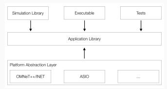
$^1\text{OMNeT}++$  model, i.e. simulated network communications  $^2\text{C}/\text{C}++$  asynchronous network library, i.e. native network communications
