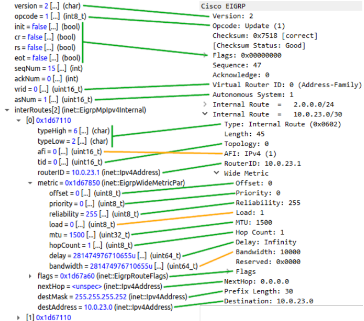
Figure 7: Scenario I - Comparison of Update message 13 from referential topology and Update message 11 from the OMNeT++ simulation.
