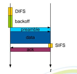
In case of IEEE 802.11g with 54 Mbps nominal capacity the attainable throughput with 1500 Byte packets is only 28 Mbps.
