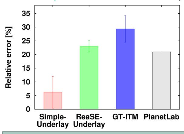
ReaSEUnderlay shows closest relative error results to real network measurements in PlanetLab
