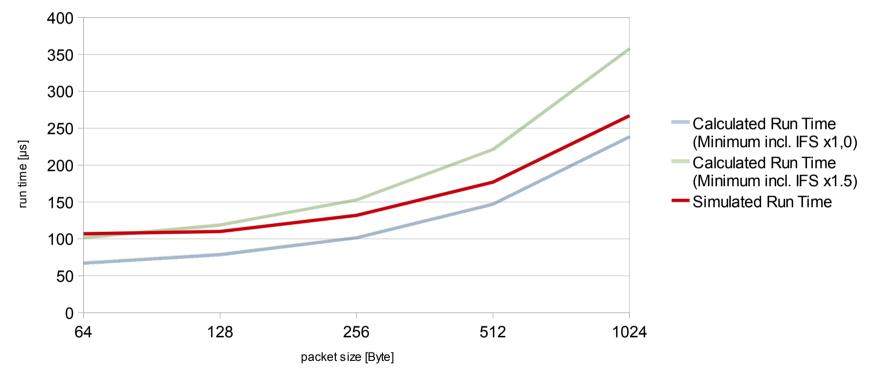
This result comes from a simple point-2-point connection network, which simulates devolo dLAN 200 modems.
