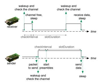
Figure 1: B-MAC protocol example with one sender and one receiver.
