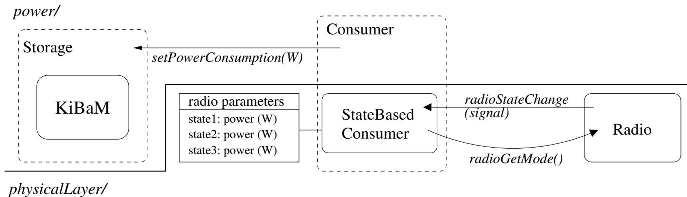
Fig. 2. Overview of the INET power framework. Power consumption is modeled by the *Consumer*, which translates information about device operations (e.g. of the *Radio*) into information about the load placed on the *Source*. Power generation is modeled using an analogous structure (not shown).
