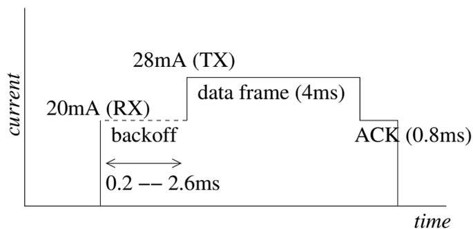
Fig. 3. Load used in simulation and in testbed experiments. Note that because the testbed provides a resistive load, rather than a constant current load, the actual current decreases over the lifetime of the experiment.
