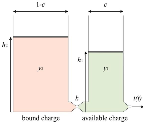
Fig. 1. Abstract view of the KiBaM model for battery state of charge.
