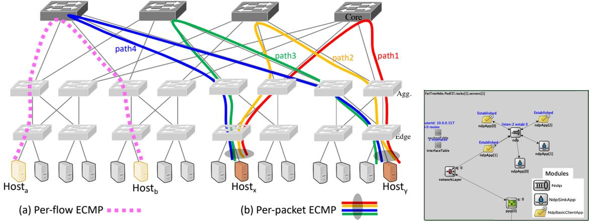
Figure 2: (a) Per-flow ECMP vs (b) per-packet ECMP in 4-FatTree
