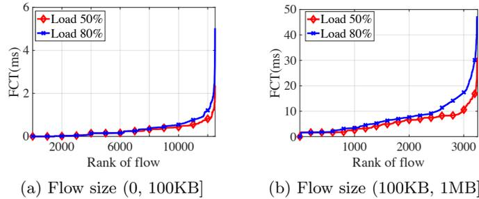
Figure 9: FCT of web search workload flows (two ranges) at different background loads
